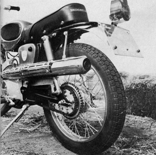
Primary drive is by helical gear to the multiplate clutch and gearbox. One rear sprocket has 34 teeth, the other 47. The engine is fed by an 1 8-mm Mikuni carburetor.
