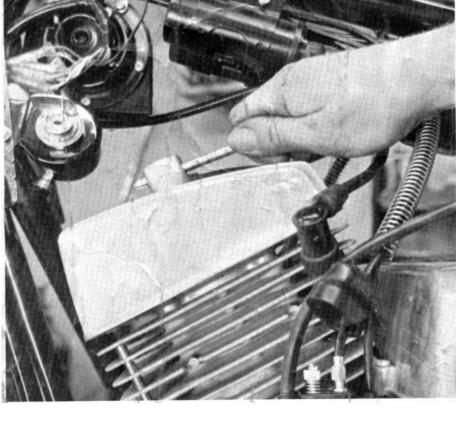
1) Since this machine is a dual rotary valve, plugs are removed and trans is put in top gear so rear wheel turns...
