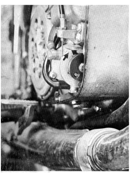
7) For timing oil pump, edge of cable pulley aligns with boss on pump when throttle slide circle touches carb orifice.
