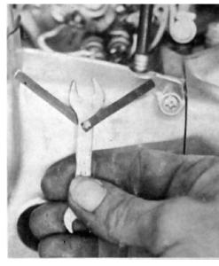
4) Set contacts at .35mm or .015-in. Wrench shown here is .3mm and .4mm so it's strictly a 'go' or 'no go' gauge.
