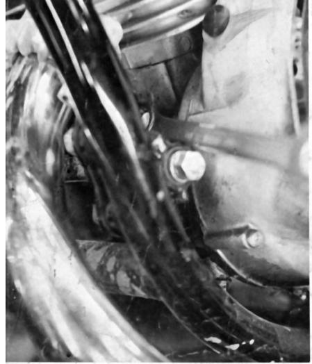
5) Remove plug in front of left cylinder and insert timing tool. A 10mm combination wrench will do the job.
