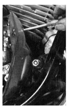
9) With carb covers installed, carbs can be adjusted externally by lifting rubber cover and turning the knurled knob.
