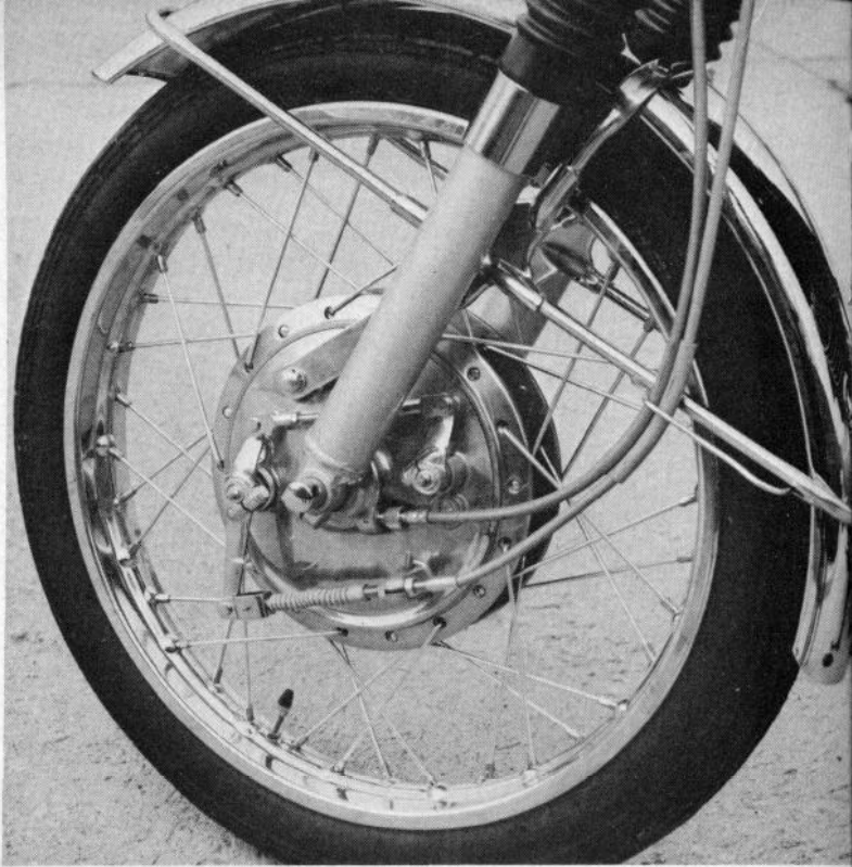
DOUBLE-LEADING shoe broke on the front wheel gives the Dual-Twin good stopping power. Steel rims mount Bridgestone tires . Springs and shocks are rubber covered. A strong brace is used on the front fender, also giving the fork extra stiffness.
